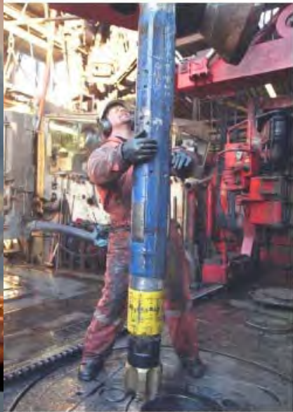
The AutoTrak rotary closed-loop system delivers higher penetration rates, more precise well placement and high-quality holes in directional and horizontal applications.
